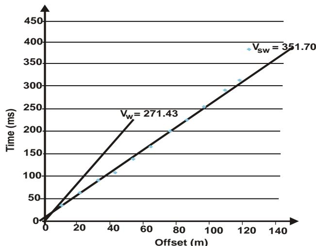
Fig. 4: Time vs Offset plot for location 3
