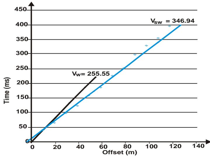
Fig. 2: Time vs Offset plot for location 1
